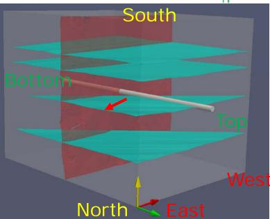
After breakdown, Fracture still propagates to East fast
